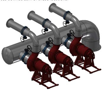
To confirm the inadequacy of the design, a Computational Fluid Dynamic (CFD) study was performed on the inlet portion of the system. The applied high flow caused large vortices to form and their proximity to the pumps was potential for catastrophic pump failure.
