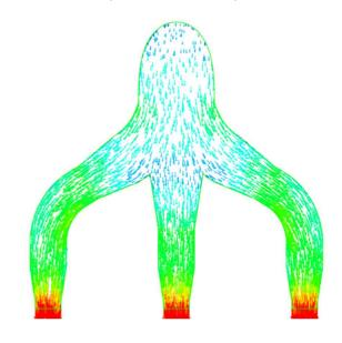
for possible swirling and were also be used to track the transport of turbulence or particle matter. Streamlines can also be integrated to provide estimations of residence time or quality of mixing if desired. Another important check made of the CFD results was the inspection of pressures which can cause cavitation acting on the pipe surfaces. In the end, a non-standard design rationalised by engineering principles was developed and verified through CFD.
